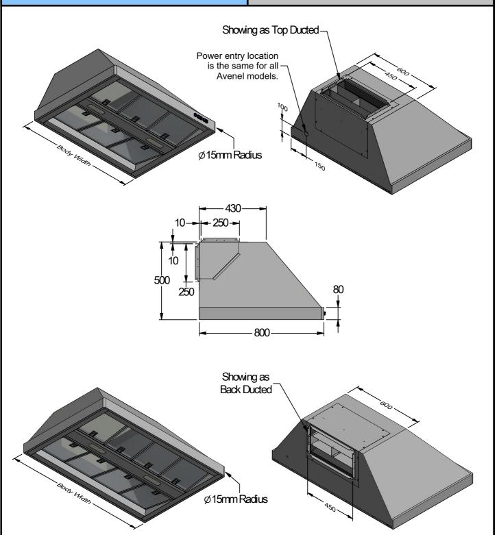
Electrical connection is made at junction box inside rangehood.
