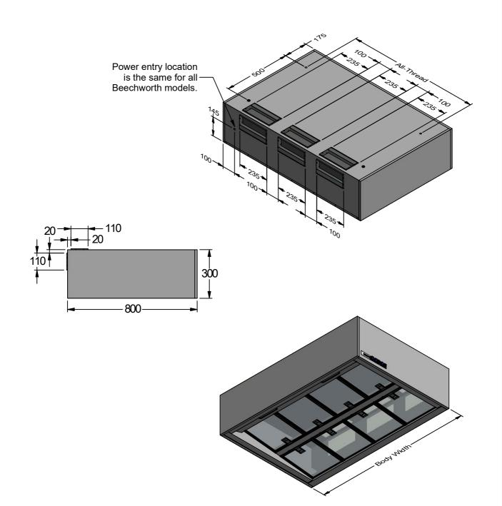
Beechworth comes top ducted and can be converted to back ducted on site by the installer. Please contact your local Qasair retailer for Ducting.
