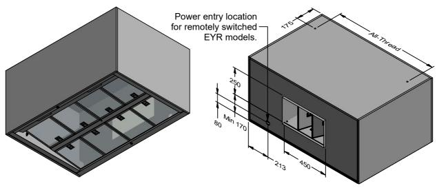
EYRE MODEL IS MADE TO ORDER AT THE REQUIRED HEIGHT AND AS EITHER TOP OR BACK DUCTED. PLEASE NOTE "R" AT THE END OF THE MODEL №. DENOTES REMOTE SWITCH FOR REMOTE SWITCH MODELS SWITCHING IS NOT SUPPLIED ELECTRICAL CONNECTION IS MADE AT JUNCTION BOX INSIDE RANGEHOOD
