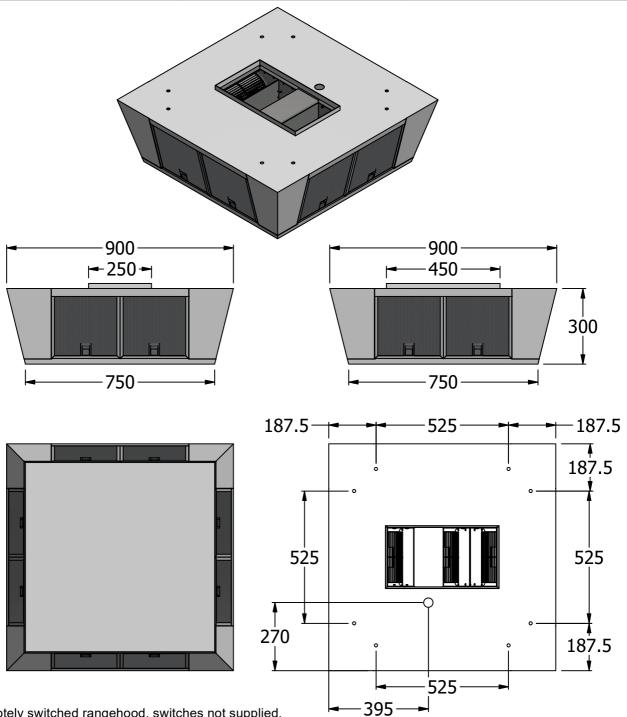
This is a remotely switched rangehood, switches not supplied. Electrical connection is made at junction box inside rangehood.
