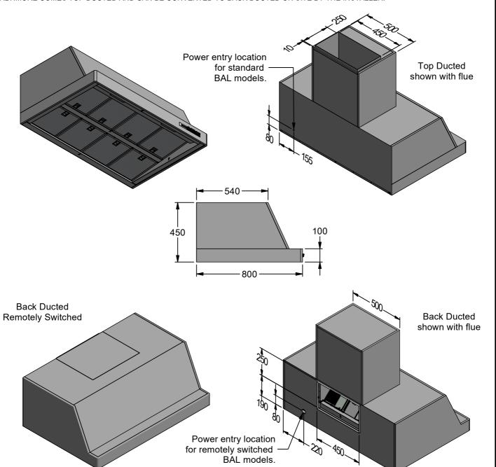
PLEASE NOTE "R" AT THE END OF THE MODEL No. DENOTES REMOTELY SWITCHED FOR REMOTELY SWITCHED MODELS SWITCHING IS NOT SUPPLIED ELECTRICAL CONNECTION IS MADE AT JUNCTION BOX INSIDE RANGEHOOD
