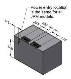
**REMOTE SWITCHED MODEL (Back Ducted Shown)**For gas / elec the recommended installation height is 650mm - 800mm. For indoor compliant open flame grill the recommended installation height is 800mm.
