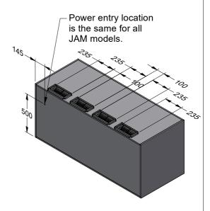
**REMOTE SWITCHED MODEL (Back Ducted Shown)**For gas / elec the recommended installation height is 650mm - 800mm. For indoor compliant open flame grill the recommended installation height is 800mm.
